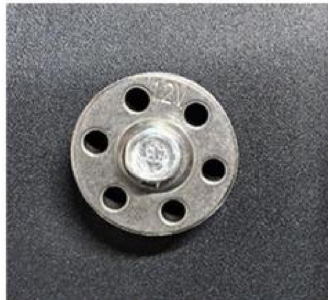
Wire feeding wheel V-shaped v1.2
