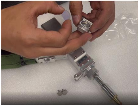
3.Replace protective lenses
